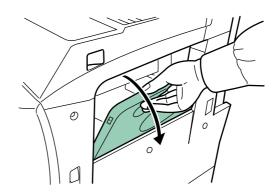
2 Remove the filters from the printer. Press in the tabs on the top filter while removing it.
